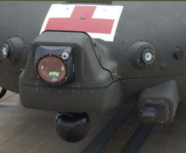
DVEPs incorporates multiple aircraft mounted sensors to provide aircrews with enhanced obstacle detection.
